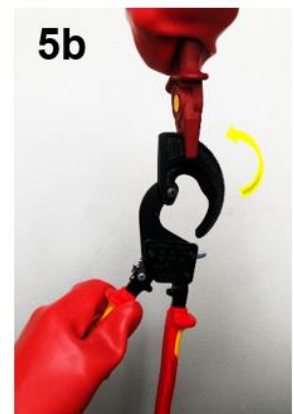
With the retaining latch (2) pressed , open the handles / allow the handles to open by spring action.
