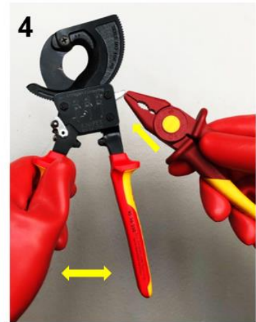
With the retaining latch (2) pressed , open the handles / allow the handles to open by spring action.
