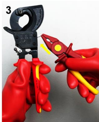
With the handles held closed, press the retaining latch (2) upwards with the insulating or hybrid pliers.
