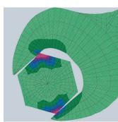
Conventional open end wrench: edge pressure causes surface damage on edges of nuts and bolts
