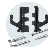
Crimping die 97 39 42: Crimps connectors for PV conductors for MC4 and MC4 Evo 2 connectors for 4 and 6 mm 2 (12 and 10 AWG)
