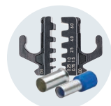
Crimping die 97 39 08: Crimps insulated and uninsulated wire ferrules from 0.25 – 6 mm 2
