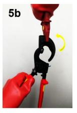
The **sickle blade (3)** is now free and can be pulled out of the cable either by pulling the cable cutter back from the cable or by pulling the sickle blade out of the cable with **insulated / insulating or hybrid pliers.**
