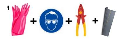
Be protected by certified insulating gloves with the appropriate insulation class for the voltage working on. Wear approved safety goggles and/or face shield.
