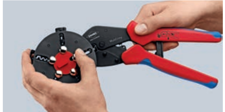
Changing the crimping dies: unlock the magazine position, take out the set of dies which the pliers have been pushed on
