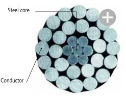
The outer area of these conductor cables consists of light, highly conductive aluminium wires, while the core is made of specially stretch-resistant, galvanized steel wires
