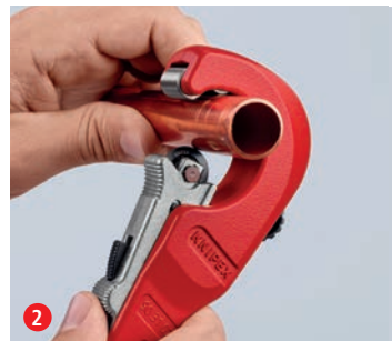
2 Push the cutting wheel against the pipe with the QuickLock one-hand locking mechanism: fastest adjustment to different pipe diameters ...
