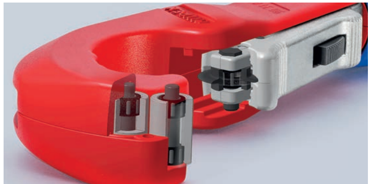
High-quality needle bearings enable the cutting wheel and the four guide rollers to operate virtually without any friction during the cutting – cuts stainless steel pipes with particular ease
