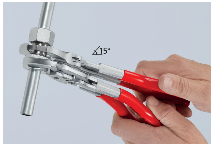
86 43 250: 15° angled pliers handle provide space for counter screw connections or bolted fittings on surfaces; reduced risk of knuckle injuries
