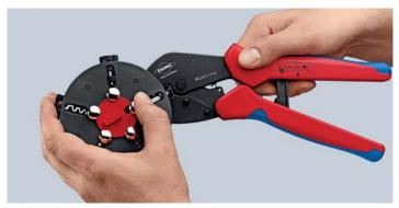
Changing the crimping dies: unlock the magazine position, take out the set of dies which the pliers have been pushed on
