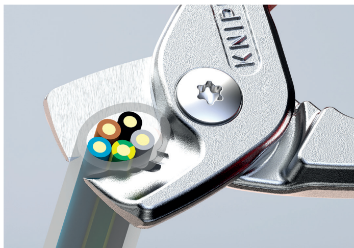
Cuts solid Cu- and Al-cable up to 5 x 4 mm 2
